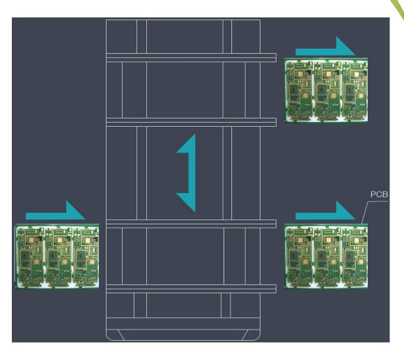
By manual lifting the conveyor section, access is gained to the rear of the line.
