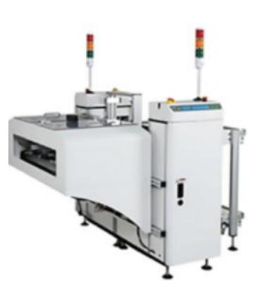
The unit loads your dual-track production line automatically by pushing PCB's out of a magazine onto the conveyor of the downstream machine.
