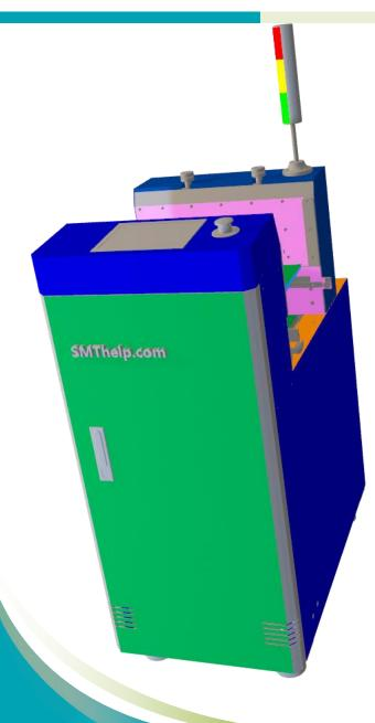
A fast, economical way to dispense bare printed circuit boards into a production line. In a double-pass line, a destack conveyor can load bare boards and a magazine unloader can introduce the second pass populated boards..
