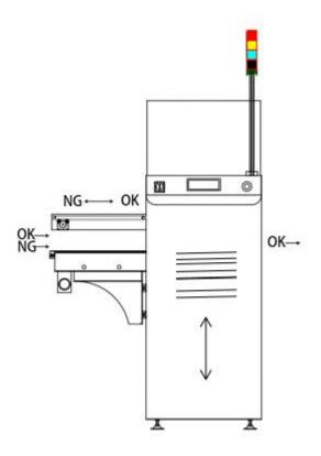
This unit is used for storage the NG board and flow to the up lever for inspection after the tester(AOI/SPI)
