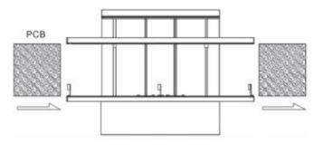
This unit is used to link between SMD machines or board handling units in dual rail PCB assembly lines.
